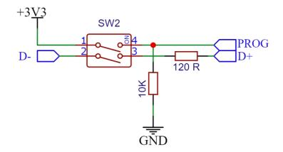
PMM0618Z can be alternatively switched between two preprogrammed modes through the second dip switch.
